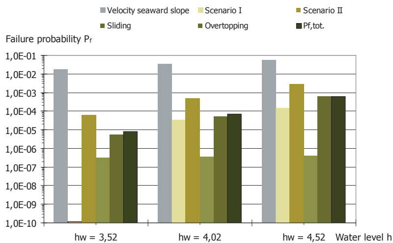
Figure 4-17: The effect of variation of the mean water level h_w on the failure probability of individual mechanisms, scenarios and overall flooding probability of the cross-section km 10,403 (Oumeraci et al., 2004).
