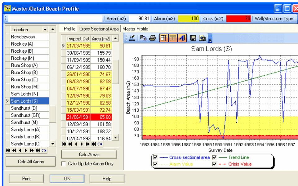
Figure 3. An example of cross-sectional area data derived from the master profile.
