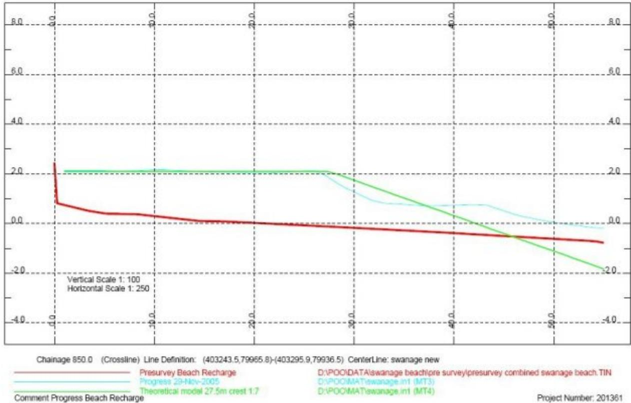
Figure 4. Example of profile survey data collected pre-survey and post-survey ([www.poolebay.net](http://www.poolebay.net), 2006).
