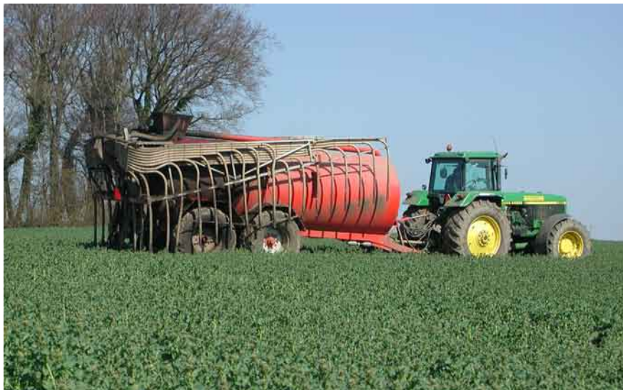
Application of slurry with trailing hoses. Photo: Bjarne Andresen.
