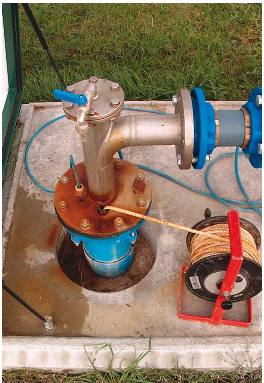
Measuring the groundwater level in a waterworks well. Photo: Peder Lerche Jensen.
