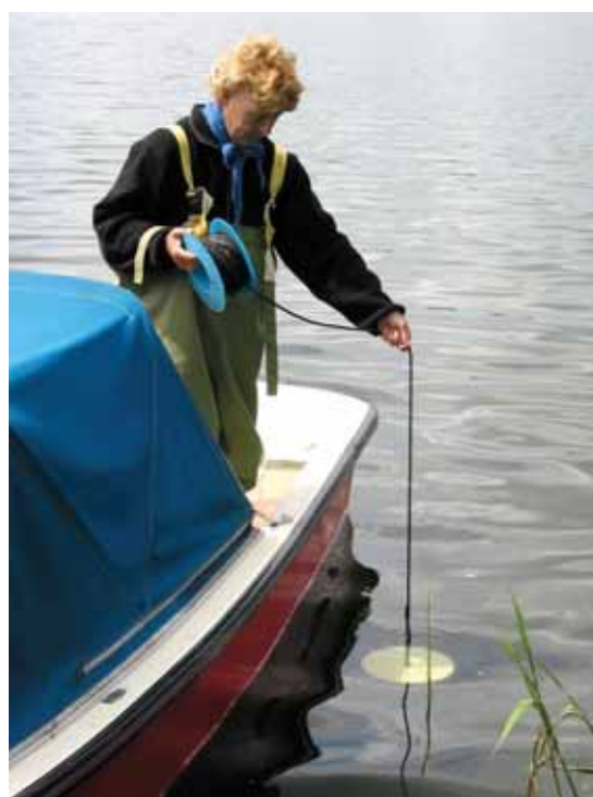
The "Secchi depth" is one of the easiest ways to characterize ecological quality in lakes. A white disc is simply lowered to the depth where it can no longer be seen. High biomasses of phytoplankton due to excess of nutrients result in low Secchi depth values and thus turbid water; low biomasses result in clear water and high Secchi depth, permitting the growth of submerged macrophytes. Photo: Jette Christiansen, Fyn County.
