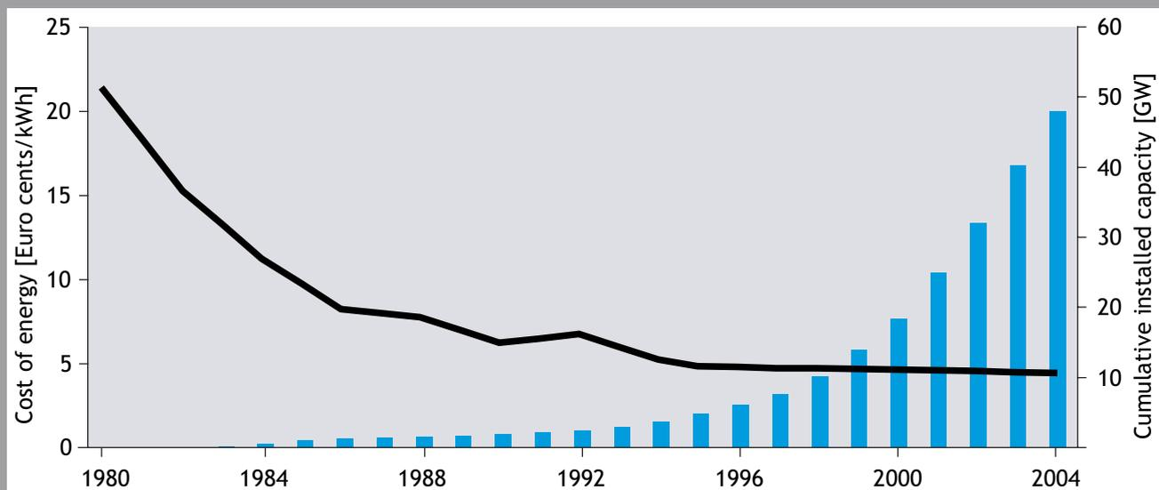
Note: The bars show worldwide cumulative installed capacity and the line indicates costs of energy.
