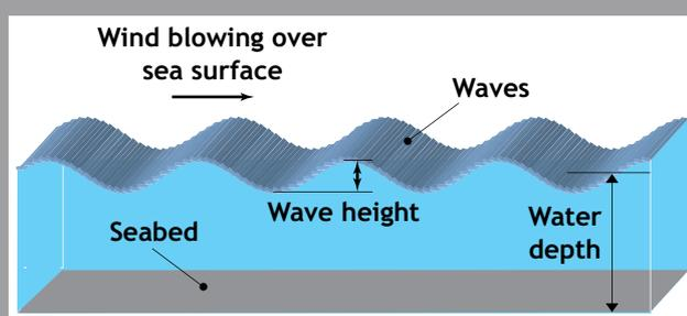
Wave energy occurs in the movements of water near the surface of the sea. Waves are formed by winds blowing over the sea surface, and the water acts as a carrier for the energy. The amount of energy in waves depends on their height and period (the time between successive peaks). The annual average power per unit length of wave crest (e.g. 40 kW/m) is a first indicator of how energetic a particular site is.
