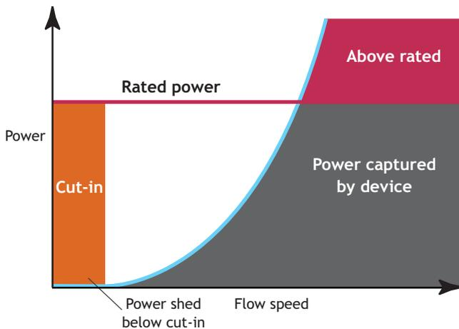
Notes: These graphs indicate ranges of operating conditions for wave energy converters and tidal stream energy generators. They are for illustration only, and neither represents a specific device technology. In each graph, the grey area shows where power would normally be generated. The orange area highlights conditions where there is insufficient energy in the resource to generate economically, and the red areas where the available energy is at or above the rated capacity of the generator.
