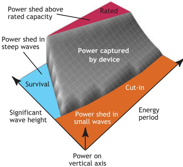
b) Example tidal stream energy generator power curve
