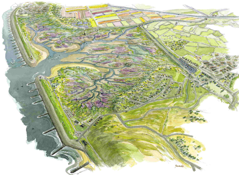
Figure 4.2: The Hondsbossche sea wall along the Dutch coast. By breaking through the sea wall, part of the land behind it will flood with the tides. The silt caught up in the vegetation ensures that the land gradually increases in height in line with or even above sea level (Drawing by Jeroen Helmer).
