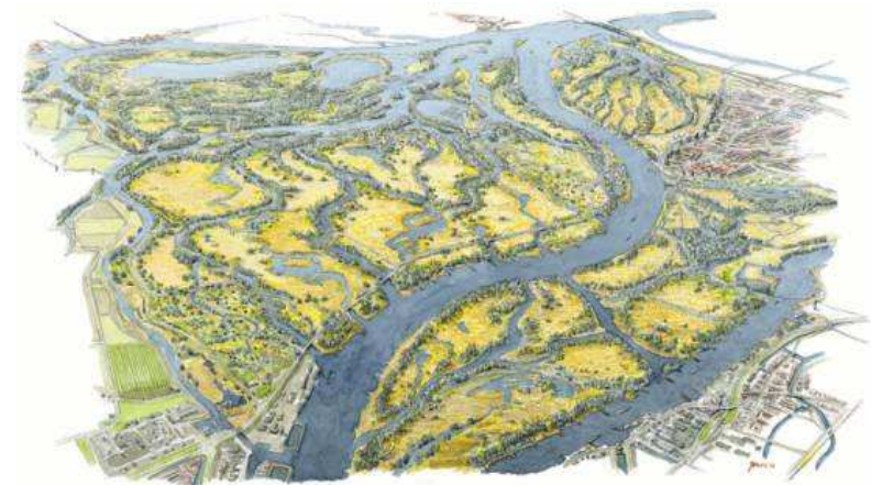
Figure 4.3: In the region around the Biesbosch, a former freshwater tidal marsh in the Netherlands, there is sufficient space to create such a storage area, thus enabling drainage peaks in the Rhine and the Meuse to be leveled off (Drawing by Jeroen Helmer).
