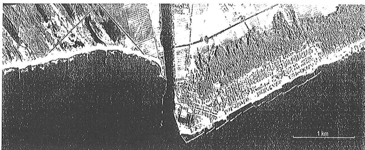
Figure 1: Arno River delta: the segment on the left eroded for 1300 m since mid 19 th century and was recently protected with groins with submerged extensions; the left side is protected by detached breakwaters facing the seawall at Marina di Pisa and by improvised structures on the downdrift sectors.
