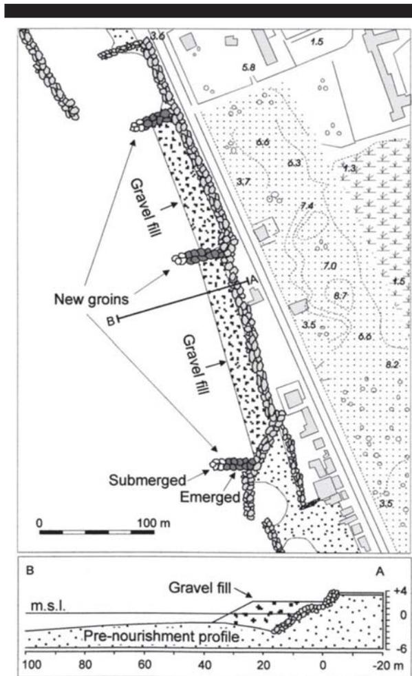
Figure 3. Design of beach nourishment project in 330 m study site (A-B profile vertical exaggeration 1:2).
