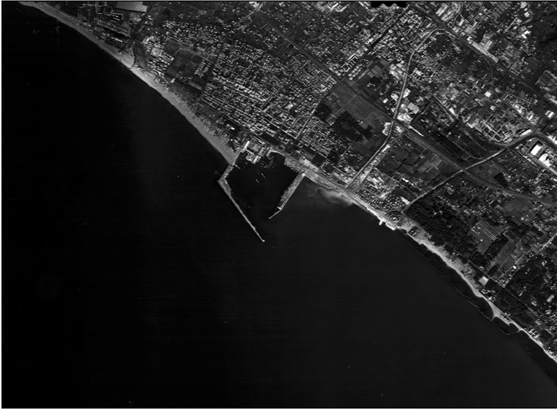
Fig 2: Marina di Carrara: beach accretion updrift the harbour is evident, as well as the downdrift erosion.
