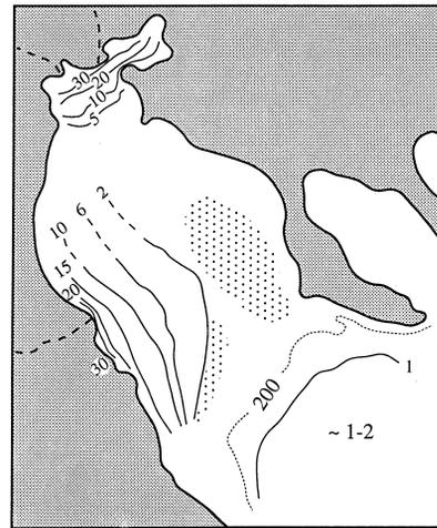
Fig. 18. Isopleths of deltaic accumulations within the Holocene, in the Thermaikos Gulf Coastal System (after Lykousis and Chronis, 1987).
