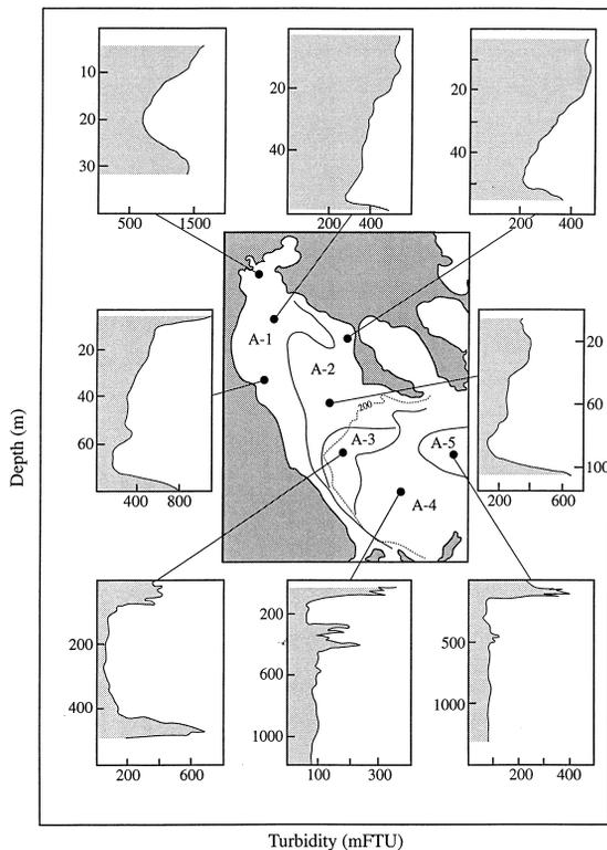
Fig. 16. Regions of relative presence of surface, intermediate and near bed nepheloid layers (after Chronis et al., 1987), with representative profiles of suspended matter (transmissometry) from Thermaikos Gulf and the adjacent Sporades Basin [Note 100–200 mFTU  $\cong$  0.3 mg/l].
