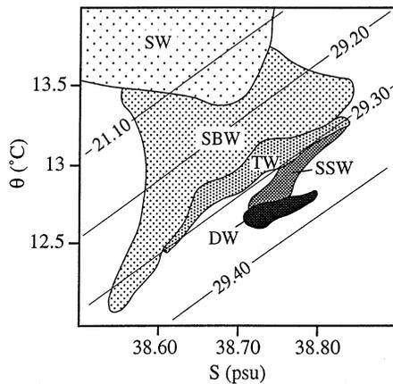
Fig. 11. Temperature (potential)–salinity diagram of the different water masses of Thermaikos Gulf (after Durrieu de Madron et al., 1992). [Key: SW: surface waters; SBW: shelf bottom waters; TW: transitional water mass; SSW: sub-surface water mass; DW: deep-water mass].
