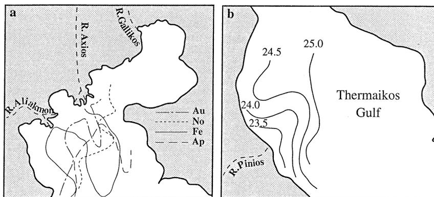
Fig. 15. River plume dispersion seawards: (a) the river mouths of the Axios, Aliakmon, Gallikos, based upon the seasonal pattern of the salinity contour of 34 psu (modified from Poulos et al., 1996a,b); and (b) the mouth of R. Pinios, as shown by the isopycnal contours (after Balopoulos et al., 1993). [Key: Au: August; No: November; Fe: February; and Ap: April].
